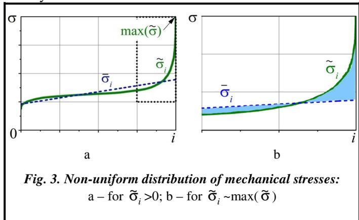
Fig. 3. Non-uniform distribution of mechanical stresses:
