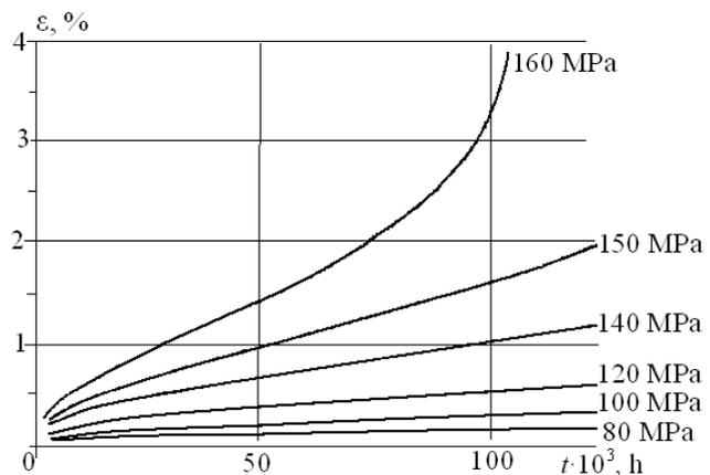
**Fig. 4. Creep curves of the diaphragm material**
