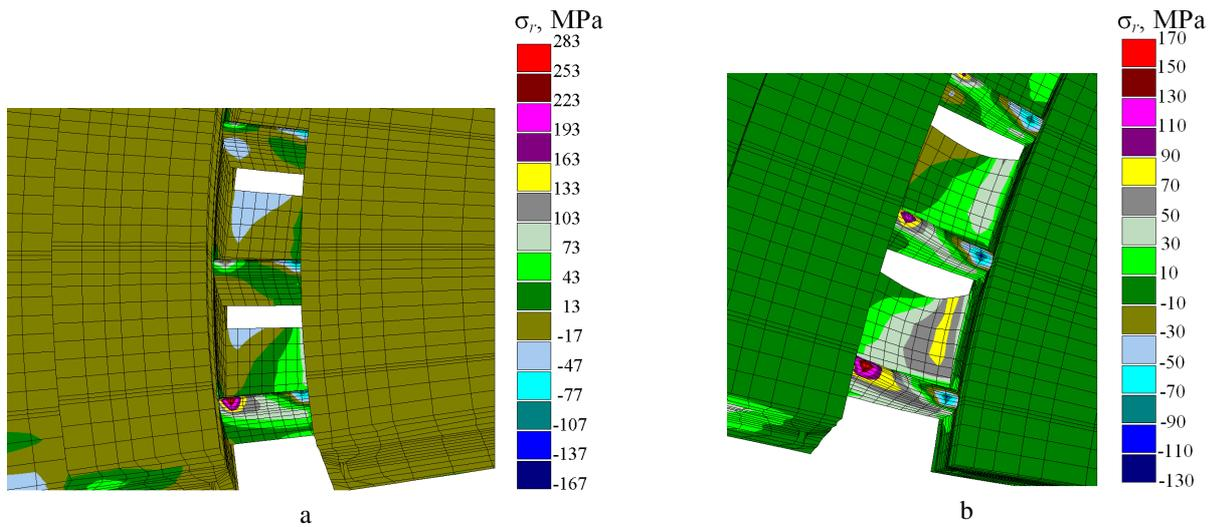
Fig. 8. Radial (along the guide vanes) stresses in the diaphragm guide vanes near the joint face: a – in the elastic state; b – during creep
