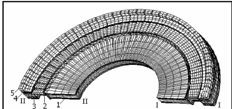
**Fig. 3. Finite element model of the diaphragm:**
