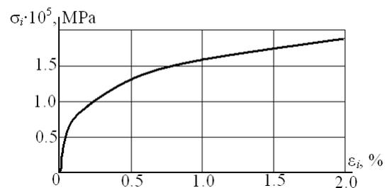
**Fig. 5. Isochronous curve for the 15H11MF steel at a temperature of 503 °C for 10<sup>5</sup> operating hours**
