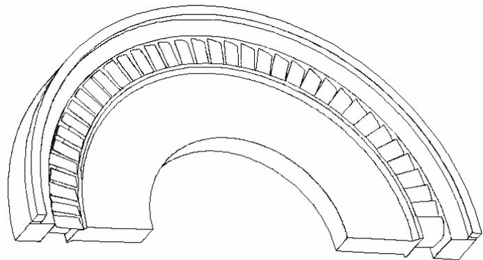
Fig. 1. Structural diagram of a steam turbine diaphragm
