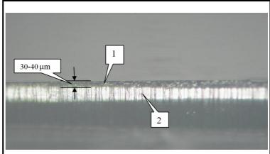
Fig. 1. The surface layer of sheet glass with cracks: 1 – surface layer microcracks; 2 – traces of macrocrack stoppage on the fracture surface of a glass sample during bend testing [6]
