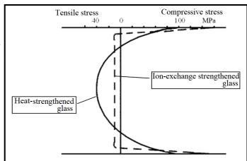
Fig. 2. Schematic representation of the in-depth distribution of compressive stresses for thermally and chemically strengthened float glass [6]
