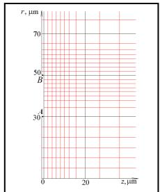
Fig. 5. Discretization of the domain into finite elements in the crack region
