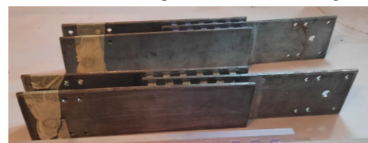
Fig. 3. Samples for the shear testing of the PLA-based HC (top) and the ULTEM 9085-based one (bottom)
