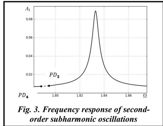
Fig. 3. Frequency response of second-order subharmonic oscillations
