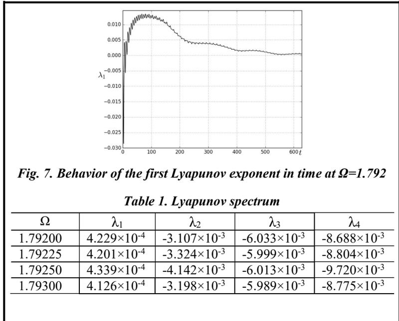
Fig. 7. Behavior of the first Lyapunov exponent in time at  $\Omega=1.792$
