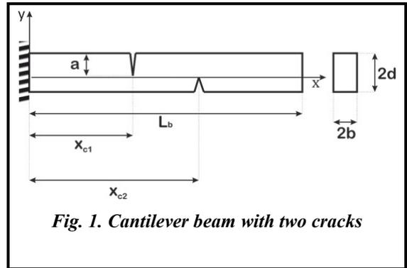
*Fig. 1. Cantilever beam with two cracks*
