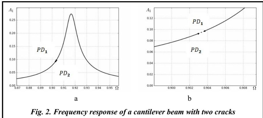
Fig. 2. Frequency response of a cantilever beam with two cracks
