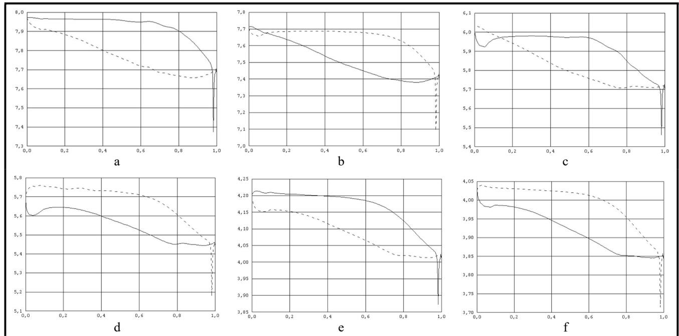
**Fig. 10. Static pressure distribution on the blade surfaces along the middle cross-section:**
