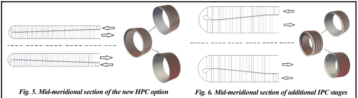
The new HPC option contains 16 reactive-type stages, as well as the additional 10 reactive-type IPC stages. Blades of all stages are designed with a constant height cross-section. The loop scheme allows to reduce the axial size for the same number of stages by almost half. From Fig. 7 it is clear that the new turbine will fit into the existing axial dimensions.
