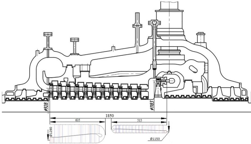
**Fig. 7. Comparison of the geometric dimensions of the existing HPC with the new HPC and IPC (the proportions in the figure are not maintained)**
