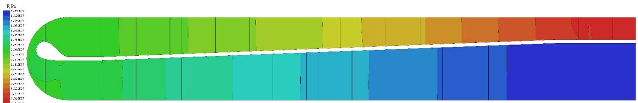
**Fig. 9. Isolines of static pressure in the HPC mid-meridional section**
