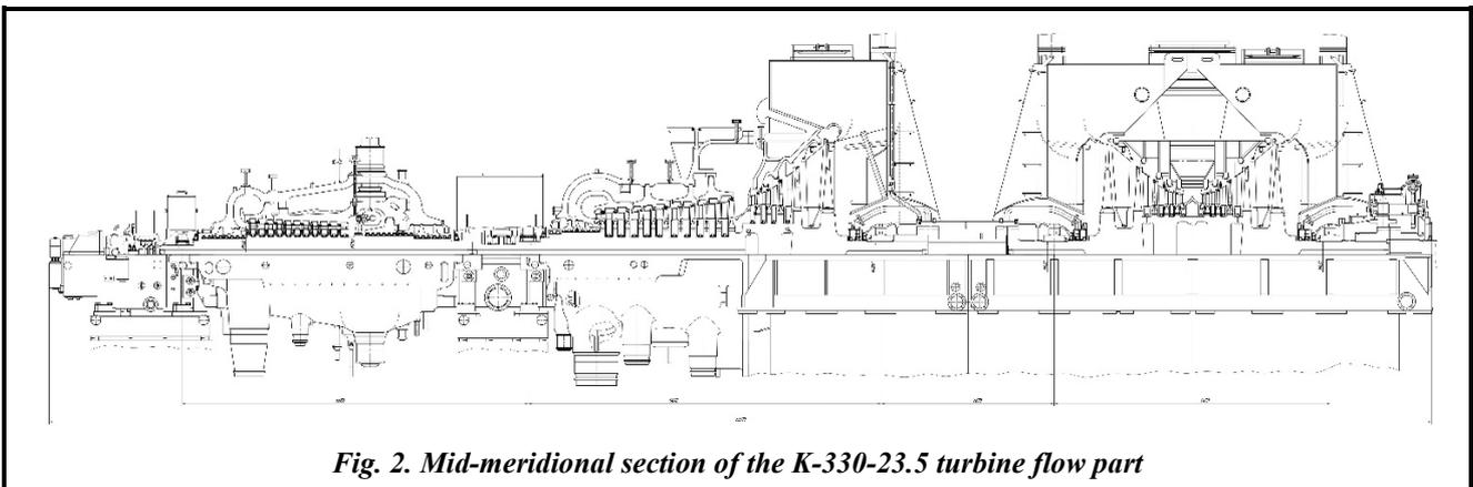
Fig. 2. Mid-meridional section of the K-330-23.5 turbine flow part
