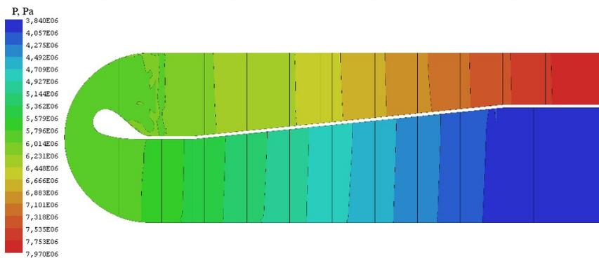
**Fig. 11. Isolines of static pressure in the additional IPC mid-meridional section**
