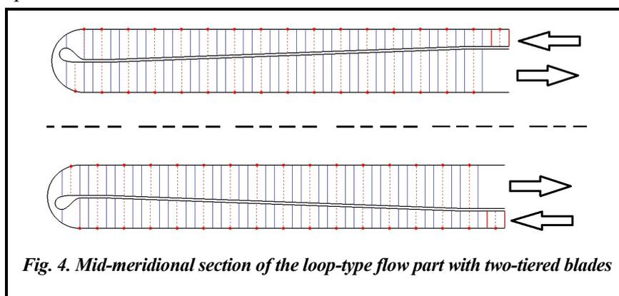
Fig. 4. Mid-meridional section of the loop-type flow part with two-tiered blades
