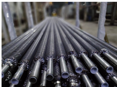
Fig. 4. General view of the finned tubes of the gas cooler
