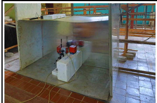
Fig. 17. A solid passive shield, in which the side surfaces of the passive shield are covered with aluminum sheets
