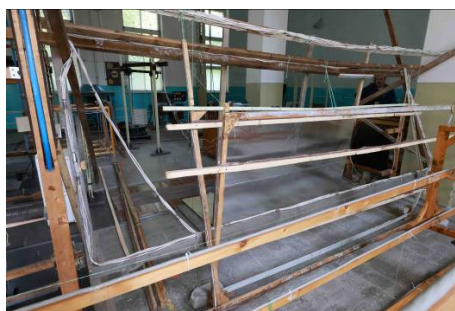
Fig. 3. Two compensating windings of the active shielding system
