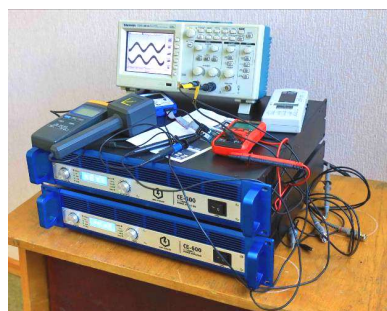
Fig. 4. Power amplifiers for powering compensating windings and measuring and recording devices
