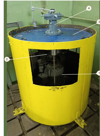
Fig. 2. General view of a pendulum semi-automatic machine for vibration-centrifugal hardening: 1 – engine; 2 – unbalanced shaft; 3 – workbench; 4 – experimental device
